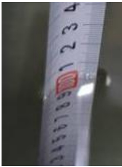
1 m Depth from The Bottom of Chamber to Water Surface
