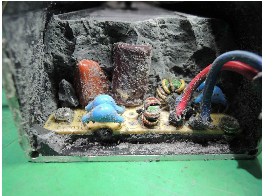
Internal View 1 of Model FSP120-FZAE1(230)MG after IP6X Testing
