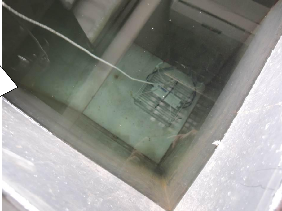
View of Model FSP120-FZAE1(230)MG under IPX7 Testing
