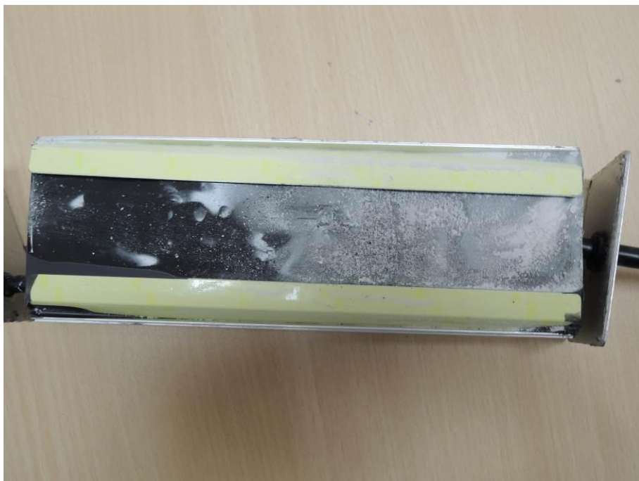
View of Dust Found on Outer Box and Internal Potting Compound of Model FSP120-FZAE1(230)MG after IP6X Testing
