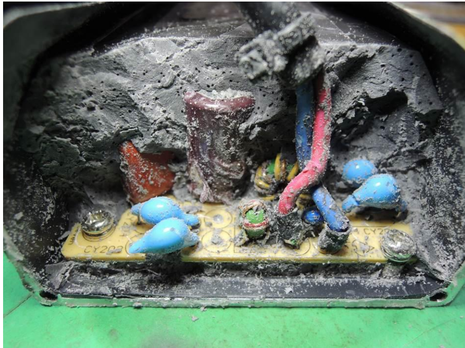
Internal View 2 Model FSP120-FZAE1(230)MG after IPX7 Test
