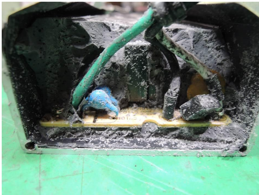
Internal View 3 of Model FSP120-FZAE1(230)MG after IPX7 Test
