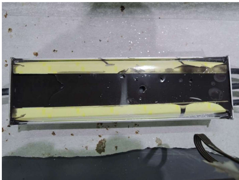
Internal View 1 of Model FSP200-FZAE1(105)DG1 after IP6X Testing
