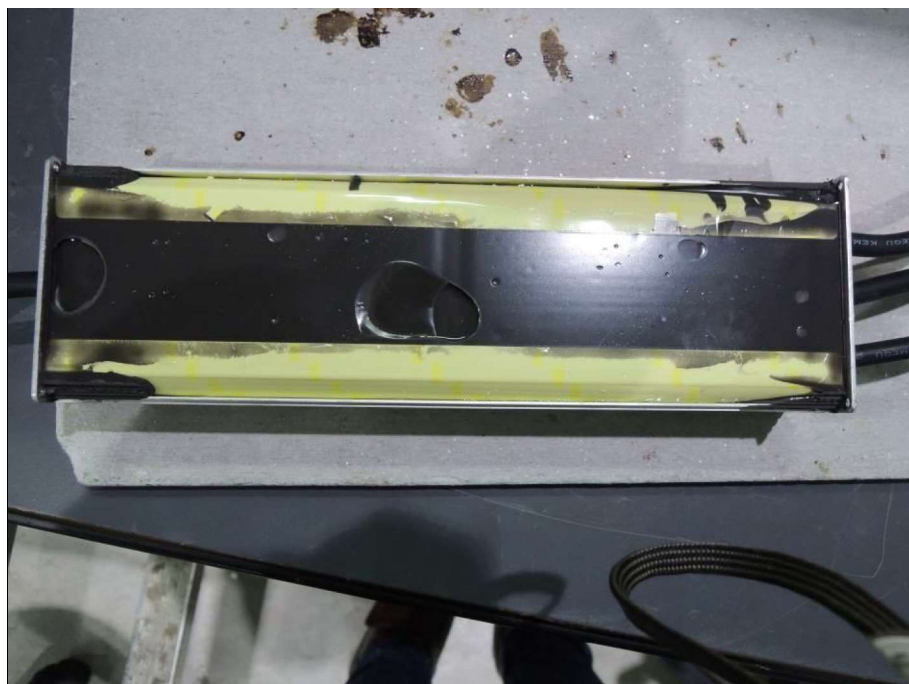
Internal View 1 of Model FSP200-FZAE1(210)DG1 after IPX7 Testing
