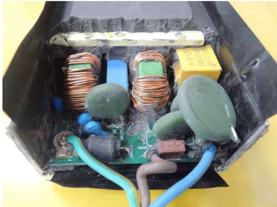
Internal View 2 of Model FSP150-SZAE(070)DG1 after IP6X Testing
