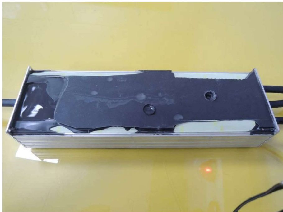
Internal View 1 of Model FSP150-SZAE(070)DG1 after IP6X Testing
