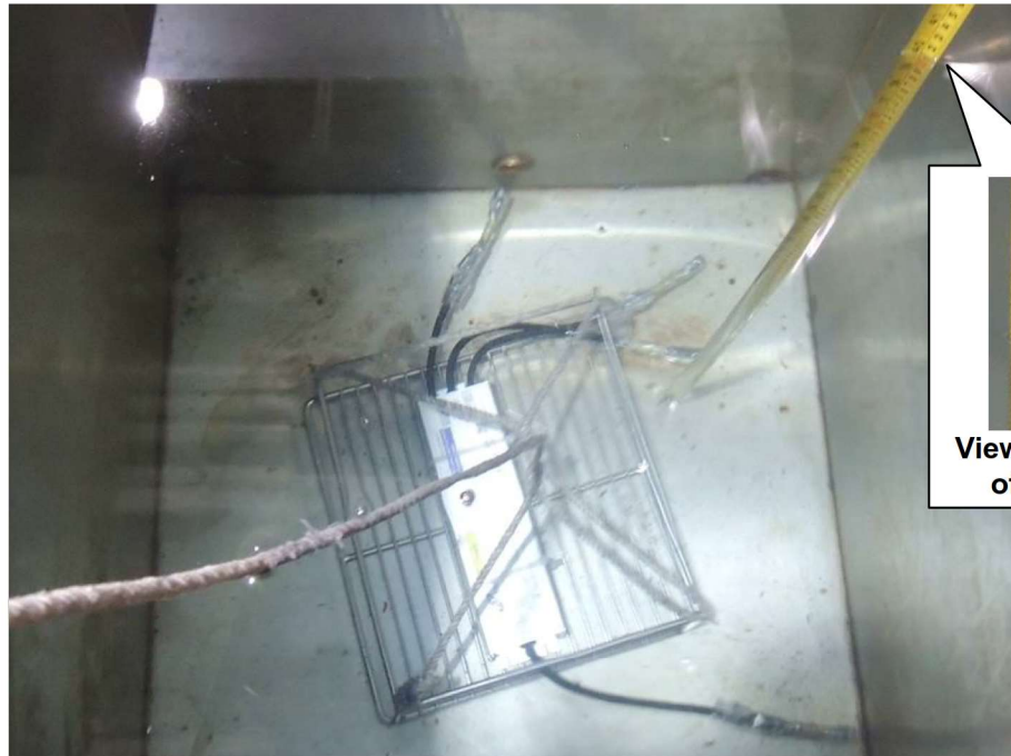
View of Model FSP150-SZAE(070)DG1 under IPX7 Testing
