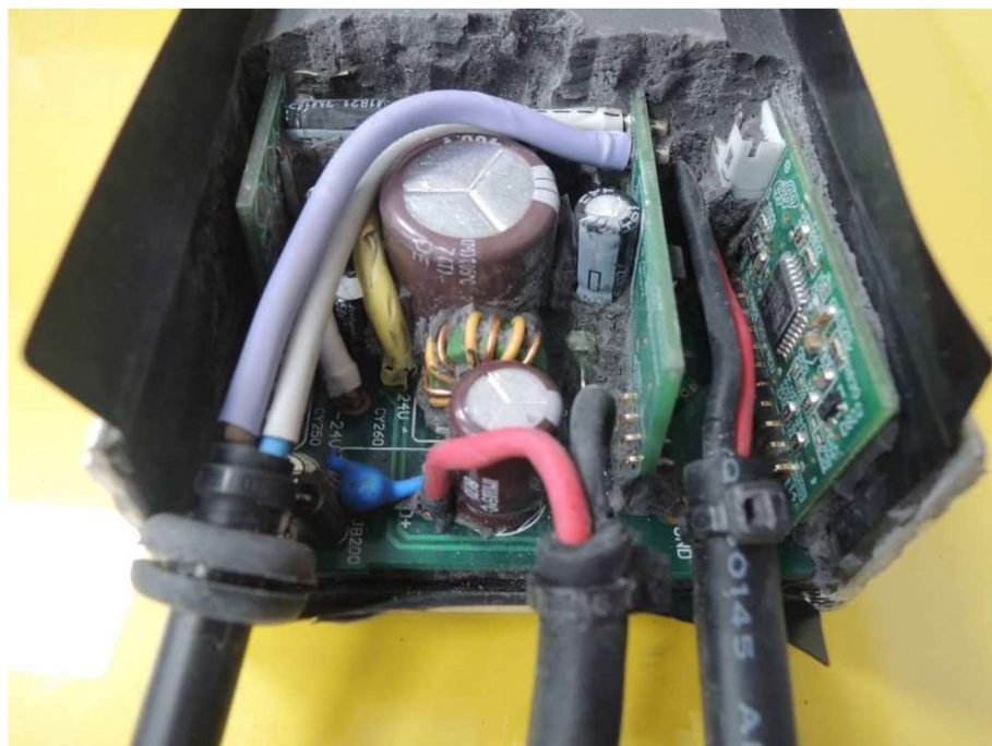
Internal View 3 of Model FSP150-SZAE(070)DG1 after IP6X Testing
