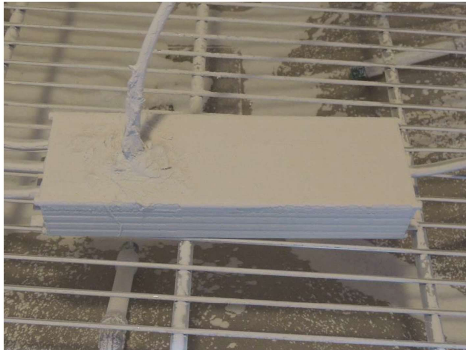
View of Model FSP150-SZAE(070)DG1 under IP6X Testing
