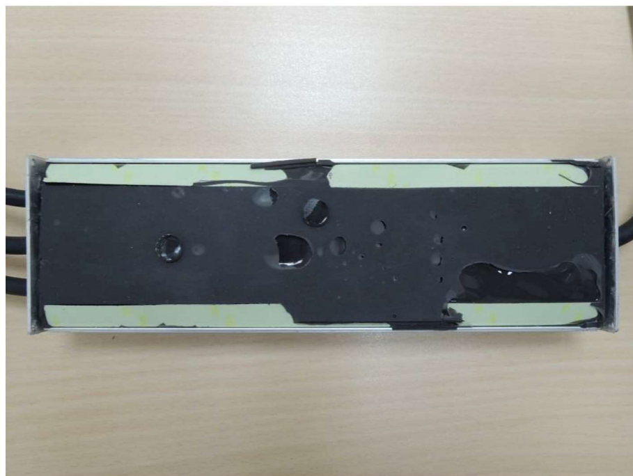
Internal View 1 of Model FSP150-SZAE(070)DG1 after IPX7 Testing
