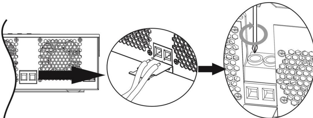
6. To firmly secure wire connection, you may fix the wires to strain relief with cable tie.
