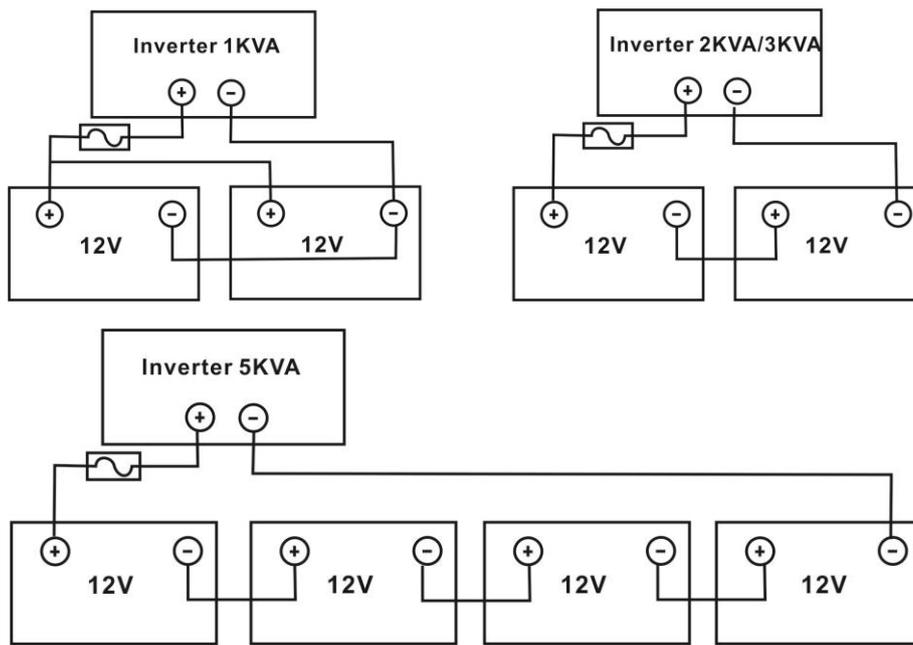
5. Insert the battery wires flatly into battery connectors of inverter and make sure the bolts are tightened with torque of 2 Nm in clockwise direction. Make sure polarity at both the battery and the inverter/charge is correctly connected and conductors are tightly screwed into the battery terminals.
