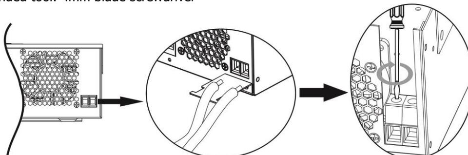
5. To ensure wires are securely connected, you fix wires to the strain relief with cable tie.
